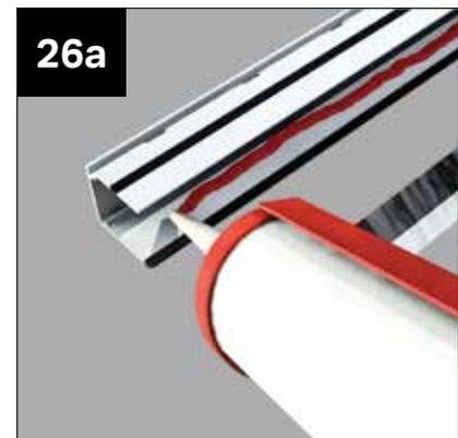
Using MS polymer seal underside of top face of glazing end profile as shown. Depending on the roof specification this can either be a PVCu or Aluminium profile. The end profile is square cut and to be aligned flush with the glazing.
