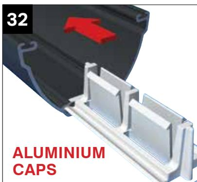
This stage should have been prepped in the factory. If not take the aluminium top caps and lay them onto a protected surface. Slide clips into each bar - position down from ridge at a max centre of 100mm and then at 500mm centres (max) inbetween.
