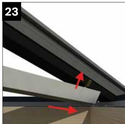
Slide undercladding down towards rider rail as far as you can and push onto clips. Hip claddings are asymmetric. Fit with short cut between hips as shown, claddings have red and blue coloured dots attached to indicate position - always use a red and blue dot at each ridge end.
