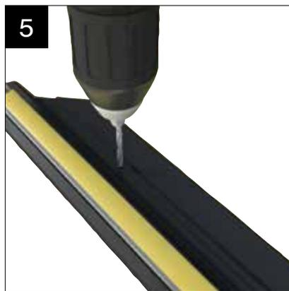
Drill the rider rail at 100mm from each end and drill a minimum of 4 holes at a Max of 400mm centres using appropriate clearance drill. Now take the rider rail and ensure correct number of bolts are slotted into rider rail.
