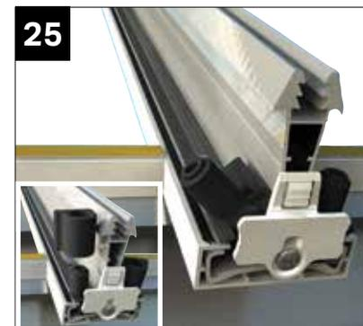
Snap off appropriate handed glazing stop (LH shown). Handing marked at base of glazing stop. Line up the rounded edge on base plate next to central web of glazing bar and tuck under gasket side of bar. Rotate glazing stop into position. Push the grommet over the post. Slide assembly down to end of bar. Repeat this for all glazing bars on the roof, excluding hip bars as these will be fit with glassLOCKS.
